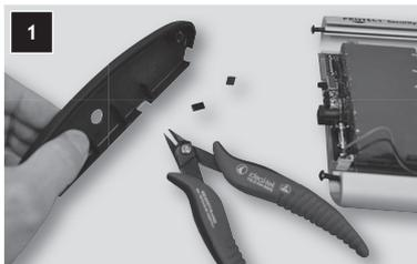
Cable access through the plastic end-caps is possible. Simply cut the prepared blankets using a sharp plier.
