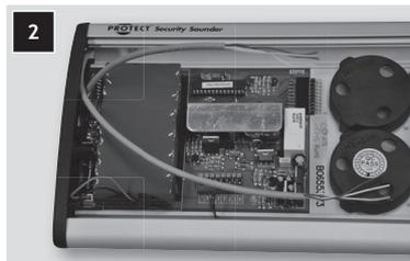
Cables shown entering the Sounder through these cable access holes.
