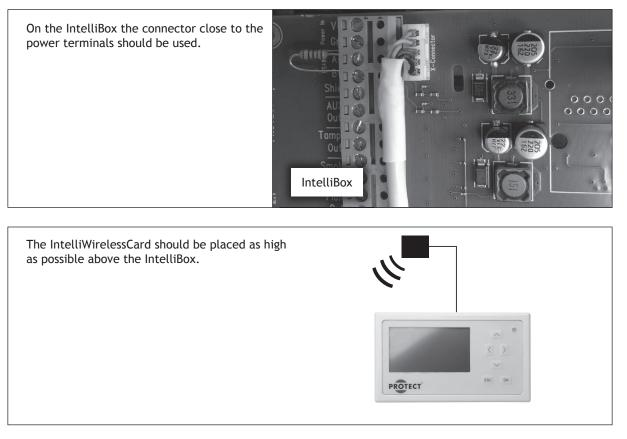
Transceivers (IntelliWirelessCards) should not be installed any closer than 2 metres from each other, since very high signal levels may overload the receivers, and hence corrupt the communication.
