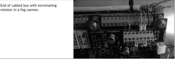
Wireless controlled fog cannon with terminating resistor.
