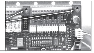
Insert and fasten the 2 spacers and washers, as shown in the picture. Plug the IntelliBusCard into the main PCB and tighten it with the 2 screws.
