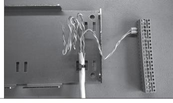
Reinstall the terminals before attaching the front to the base.
