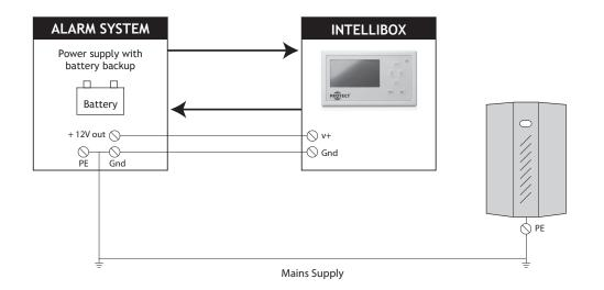
If the power supply to the IntelliBox is taken from the existing alarm system, it's GND should also be connected to earth.
