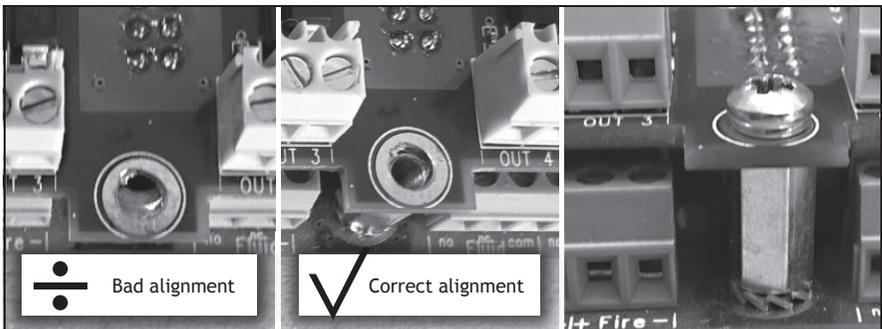
The connector on the IPCard™ MUST align properly with the connector on the main board, and mounting holes in the IPCard™ must align with spacers before attempting to install the screws.
