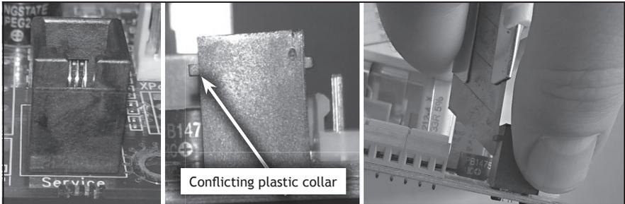
On some Fog Cannon™ units a service connector on the main PCB may have to be modified to give space enough to install the IPCard™.
