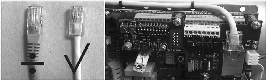
Route the networking cable as shown in the picture to make sure cable will not conflict with any internal part of the Fog Cannon™. Let the network cable exit the hole in the cabinet used for any other normal signal cable to and from the alarm system.
