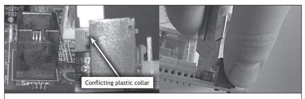
On some fog cannon units a service connector on the main PCB may have to be modified to give space enough to install the MultiCard
