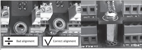
The connector on the MultiCard <u>MUST align properly</u> with the connector on the main board, and mounting holes in the MultiCard must align with spacers before attempting to install the screws.
